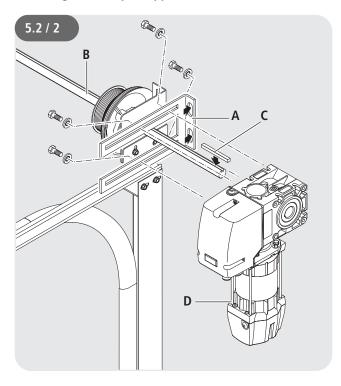
Fit the torque support bracket/console (A).
